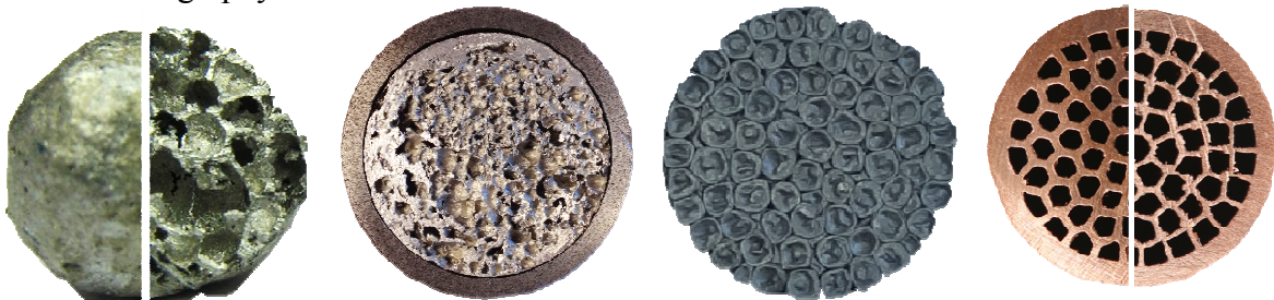
Figure 1. Different types of cellular materials.
